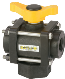
3-WAY VALVES POLYPROPYLENE BODY VITON SEALS TEFLON SEATS 100 PSI @ 72°F FPT THREADS ST. STEEL BOLTS BL=BOTTOM LOAD SL=SIDE LOAD
