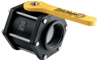
BOLTED BALL VALVES (BBV) SEALS TEFLON SEATS 100 PSI @ 72°F FPT THREADS ST. STEEL BOLTS
