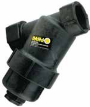
Y STRAINERS POLYPROPYLENE BODY EPDM GASKET (VITON AVAILABLE) ST. STEEL SCREENS FPT THREADS
