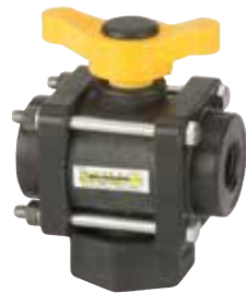
3-WAY VALVES POLYPROPYLENE BODY VITON SEALS TEFLON SEATS 100 PSI @ 72°F FPT THREADS ST. STEEL BOLTS BL=BOTTOM LOAD SL=SIDE LOAD
