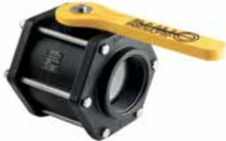
BOLTED BALL VALVES (BBV) SEALS TEFLON SEATS 100 PSI @ 72°F FPT THREADS ST. STEEL BOLTS
